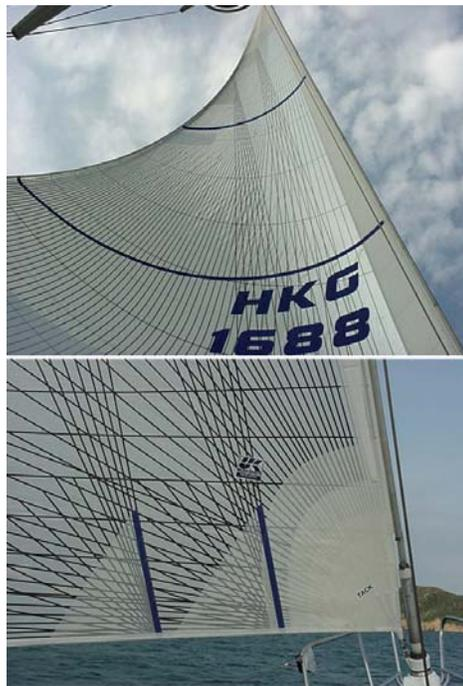
*These pictures show the extra tapes that carry the loads when the sail is reefed. The tapes connecting the reef reinforcements on the foot and the leech also make it easier to roll the sail up to a reef point.*
